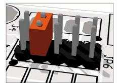
JP6 Pin 3 of the screw terminal is connected to Ethernut's signal ground via a 100 Ohm resistor (R26) and can be used to connect a cable shield. Alternatively pins 3 and 4 of the screw terminal may be used to provide power to the external RS-485 device. In this case shorten pins 3 and 4 of JP6 to disable R26 and connect screw terminal pin 3 directly to ground.
