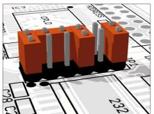
JP1 If your application requires hardware handshake via RTS/CTS, then connect JP1 pins 4 and 6 and pins 5 and 7. The picture on the right shows the hardware handshake configuration for UART0.
