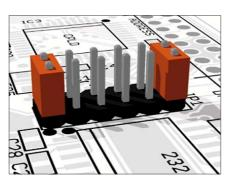
JP1 Shortening pins 1 and 2 and pins 11 and 12 will route UART0 transmit and receive lines to the DB-9 connector.
