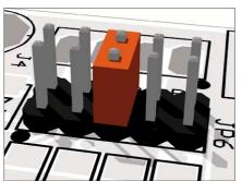
JP6 Both ends of a RS-485 communication line must be terminated by a resistor. If the Ethernut board is located at one end of the line, you must short pins 5 and 6 of JP6 to enable the 120 Ohm termination resistor (R24).
