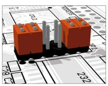
JP1 Most applications will probably use UART0 for RS-232 and UART1 for RS-485. This configuration is shown below. Pins 1 and 2, 3 and 4, 9 and 10 and 11 and 12 of JP1 are shortened.
