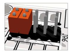
JP6 Pin 4 of the screw terminal is connected to the Ethernut's unregulated DC line via a diode (D2). The diode protects the Ethernut from supply with wrong polarity. If you want Ethernut to supply external devices, the diode must be disabled by shortening pins 1 and 2. Be aware, that this jumper bridge should only be set to supply external devices and should always be removed when supplying Ethernut via the screw terminal.
