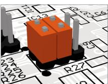
JP2 The RS-485 interface is half duplex. Only two wires are needed for communication, but an additional port bit is required to switch between receive and transmit mode. Thus pins 1 and 2 as well as pins 3 and 4 of JP2 must be shortened to control the data direction via ATmega port bit PD5.
