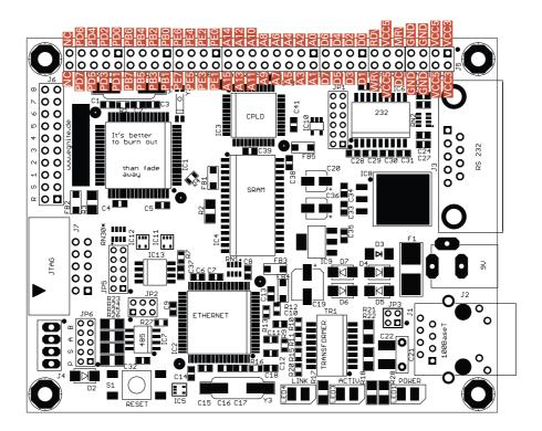
The expansion port contains CPU data and address bus, memory read/write signals, digital I/O ports, reset signal and power supply. Nearly all microcontroller pins are available at the expansion port connector, providing an interface with lots of features like PWM, I2C (2-wire), SPI (3-wire) or counter inputs, to name just a few. It is strictly recommended to consult the ATmega 128 data sheet before attaching hardware to the expansion port.
