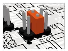
JP2 The direction signal is pulled low by R27. If pins 3 and 4 are shortened only, the RS-485 interface is configured as a receiver and no port bit for direction control is required.
