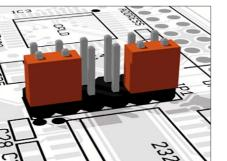
JP1 When pins 1 and 3 and pins 9 and 11 are shortened, then UART1 is connected to the DB-9 connector.
