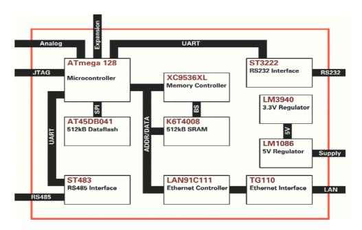
The microcontroller provides two UART channels, which are routed to the onboard RS-232 and RS-485 level shifters.
