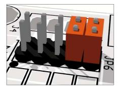
JP6 During switching from transmit to receive mode, the condition of the RS-485 line becomes undetermined and may introduce problems on connected receivers. Shortening pins 7 and 8 and pins 9 and 10 will enable two 560 Ohm fail safe resistors (R23 and R25). These resistors should be enabled on one end only.
