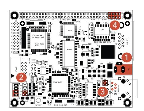
1 A standard 2.1 mm barrel connector. This input is protected by a fuse (F1), a fast transient voltage suppressor (D3) and a rectifier bridge (D4, D5, D6 and D7).
